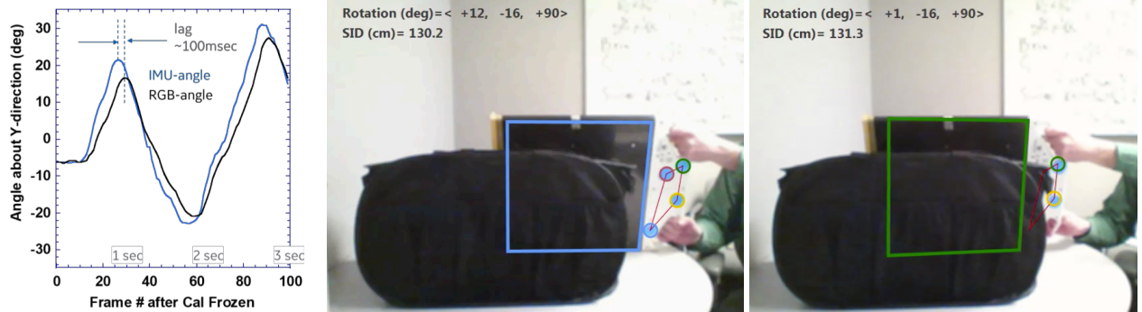
Figure 2 An IMU mounted to the detector measures three rotation angles that closely follow the camera-based angle except for a lag (left) due to acquisition and wireless communication delays; tracking of the detector 6-DOF position and rotation with the camera combined with 3-DOF rotation from the IMU can accommodate partial visual occlusion (right) of the detector in the camera's field of view.
