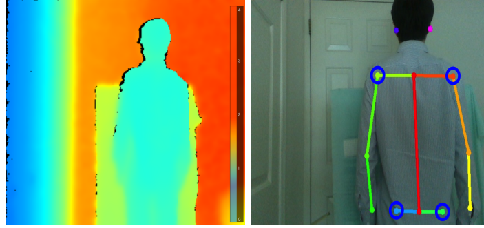
Figure 1. Depth image (left) and RGB image with detected joint keypoints (right) from D435 camera (blue annuli indicate our selected keypoints in anatomy registration).
